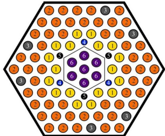
**Fig. 3.** Internal elements of the fuel assembly control unit 1 - "light" fuel element (18), 2 - "heavy" fuel element (54), 3 - burnable absorber 1 type (6), 4 - burnable absorber 2 type (3), 5 - zirconium displacer (3), 6 - compensating rods (6)
