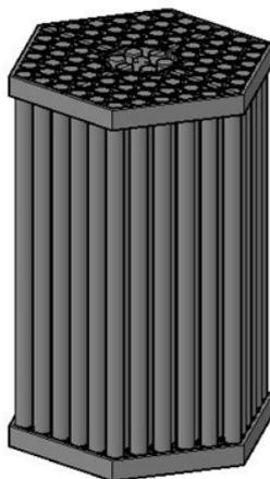
**Fig. 2.** Fuel assembly simulator
