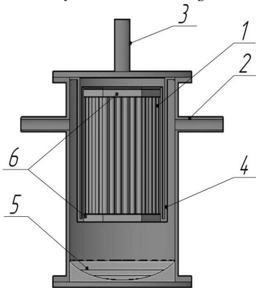
**Fig. 1.** General view of the research stand: 1 – fuel assembly simulator; 2 - pipe of the coolant inlet; 3 - pipe of the coolant outlet; 4 - shells; 5 - elliptical insert; 6 - remote grates)
