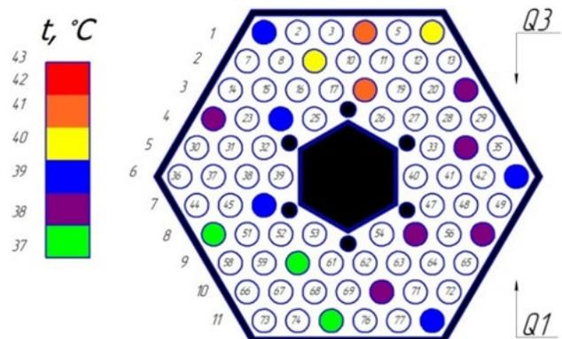
Fig. 7. Distribution of temperature at the input to the simulator active zone in dynamic mode
