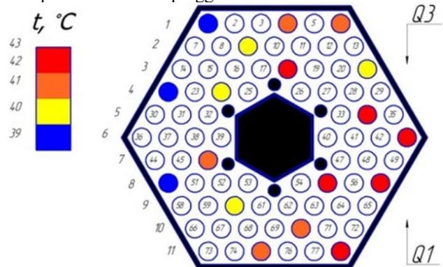
Fig. 6. Input temperature distribution of to the simulator active zone in a stationary mode
